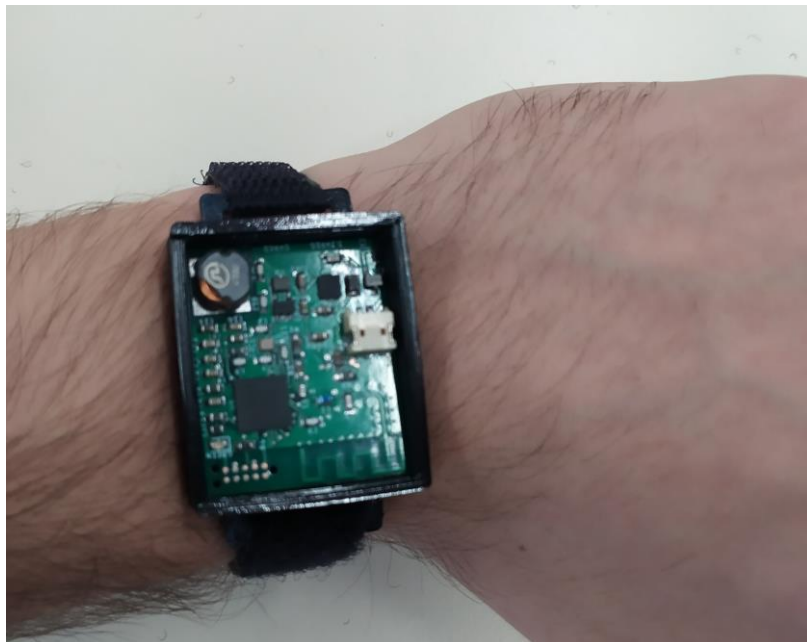
Figure 1. Digital Triage Tag. Early prototype v0.1 (Does not yet include all submodules).
