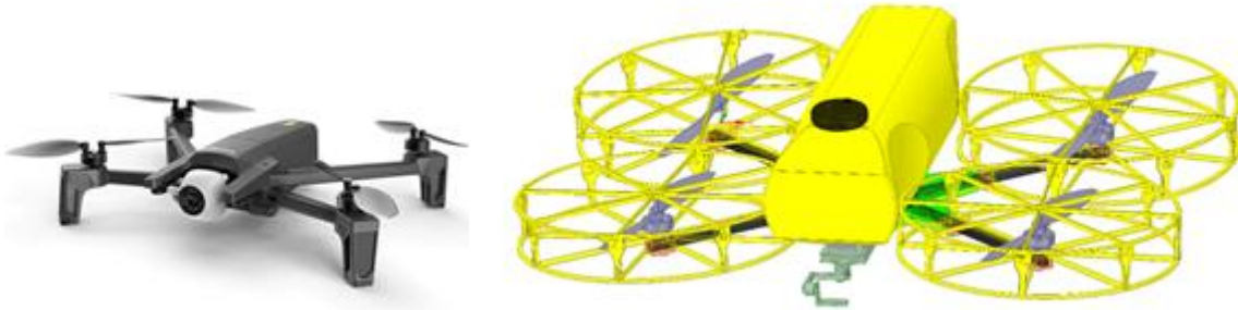
Figure 8. The drone components UAR-SAS (photograph) and UAR-TIS (design view).
