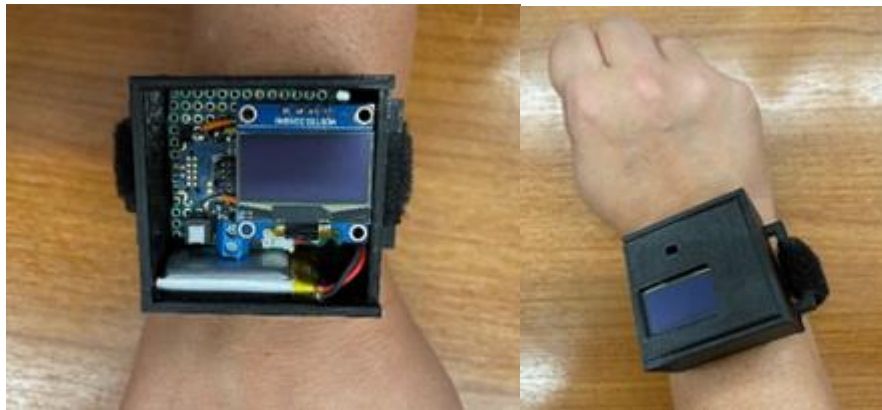
Figure 2. FR wearable. Early prototype V0.1. The final prototype dimensions are estimated to be 4,5 x 4,5 x 1,5 cm
